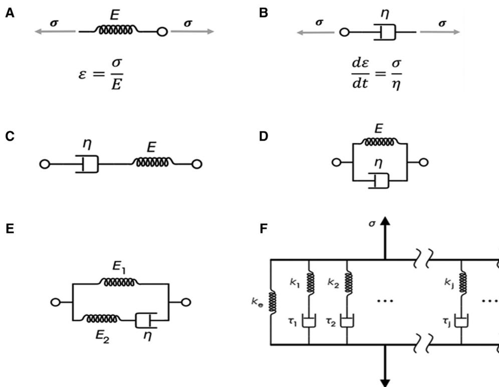
**Supplementary Fig.** Constitutive models of linear viscoelasticity: **A**, spring; **B**, damper (dashpot); **C**, Maxwell model; **D**, Kelvin-Voigt model; **E**, standard solid model; **F**, generalized Maxwell model.
