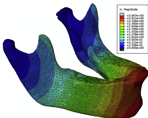
**Fig 4.** Viscoelastic modeling displacement. The symphysis area exhibits a displacement of approximately 3.067 mm. See the Video (available at [www.ajodo.org](http://www.ajodo.org)) for animation.
